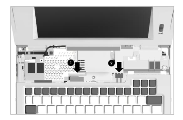
Figure 5-39. Disconnecting the Keyboard
